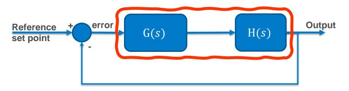
We were working with open loop transfer function  $G(s)H(s) = K \frac{N(s)}{D(s)}$
